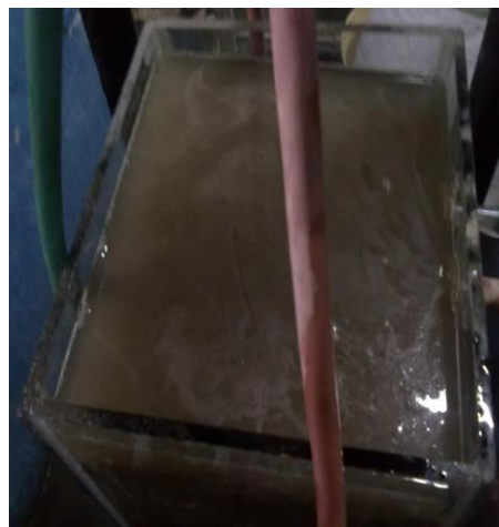
Fig 4.1: Boiling condition of the sand with 1% silt
